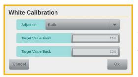
Also the White Calibration, as 2nd step of this calibration, is performed with a lower target value of **224** (default is 260). Like at the gain calibration, the value of the **Target Value Front/Back** fields is also changed here in the associated mask and saved for future calibrations from the areas **Service** and **Administration**. Then, as usual, perform the White Calibration with the paper provided for this purpose.
