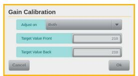
The first step is a Gain Calibration to a **Target Value** of **210** (default is 250). For this purpose, the value of the fields **Target Value Front/Back** in the corresponding mask of the **Gain Calibration** button in the menu Service-> Calibration is changed accordingly and, after inserting the white balance paper, the calibration is started with the button **OK**. The last used target value will be stored in the
