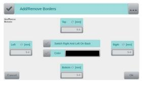
If the UTT is to be scanned with the *Deskew* option enabled, we recommend using the *Overscan function* to keep enough margin around the image to analyze the target. To do this, activate the *Add/Remove Border* item in the *Image Presettings* menu and define a value of *5 mm* on all sides in its mask. In addition, the *Color* option must be *disabled* in the center so that the original background remains as a frame.
