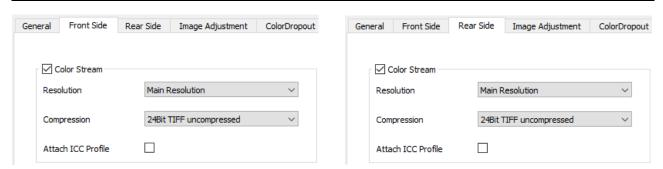
On the tabs *Front* and *Back*, the *Color Stream* must be **enabled** and the *Compression* must be set to **24Bit TIFF uncompressed**. The option *Attach ICC Profile* remains deactivated, but can be activated after creating and importing the color profiles to the scanner in order to transfer these color profiles together with the color images to the scan software.
