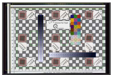
If not all points have been passed, first check if the analysis fields have been placed correctly on the image of the target. This can be done with the button Image (right bottom edge at Settings area), which switches from the Overview to the display of the target image with entered fields (called patches - see left). If there are significant divergences, either the scan of the UTT target should be repeated or the Detection can be changed to Manual Mode. The further procedure for adjusting the
