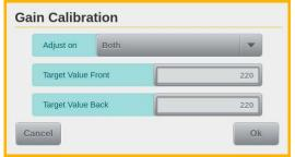
The first step is a Gain Calibration to a *Target Value* of *220* (*default is 250*). For this purpose, the value of the fields *Target Value Front/Back* in the corresponding mask of the *Gain Calibration* button in the menu Service-> Calibration is changed accordingly and, after inserting the white balance paper, the calibration is started with the button *OK*. The last used target value will be stored in the
