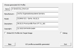
In the lower part of the dialog, the *Save* button is used to select name and path of the color profile to be created. If the color profile should be imported on the scanner later on, we recommend using the name *icc\_front.icm* for a front side profile and *icc\_back.icm* for a back side profile. Information about the color profile can be entered in the four fields below. The field *Description* is automatically filled with to the selected profile name and represents the reference used as
