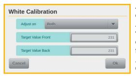
Also the White Calibration, as 2nd step of this calibration, is performed with a lower target value of **231** (default is 260). Like at the gain calibration, the value of the **Target Value Front/Back** fields is also changed here in the associated mask and saved for future calibrations from the areas **Service** and **Administration**. Then, as usual, perform the White Calibration with the paper provided for this purpose.
