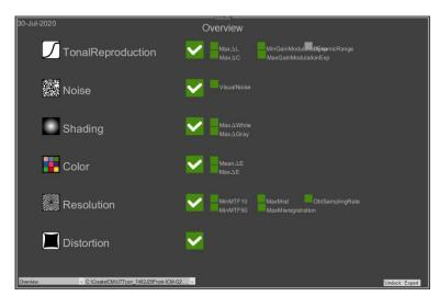
Once the image analysis has been completed, an *Overview* appears in the main screen of the application, ideally showing green checkmarks in all six checked points (figure left). This means that the points have been passed the tests of the selected specification. If one or more points show a red cross here, the specification were not met in the corresponding kind of test.
