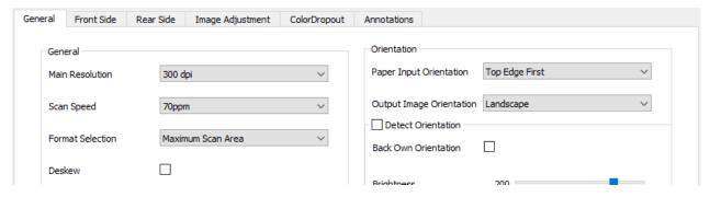
In the *General* tab, the required *Main Resolution* (here **300 dpi**) and a *Scan Speed* of **120 ppm** or (with Slow Mode option) even slower should be selected. At Format Selection, **Maximum Scan Area** must be selected and **Landscape** for *Image Output Orientation*. The Paper Input Orientation depends on the UTT format used. Select **Top Edge First** for A4 and **Right Edge First** for A3. Whether **Deskew** is activated or not should depend on the productive use.
